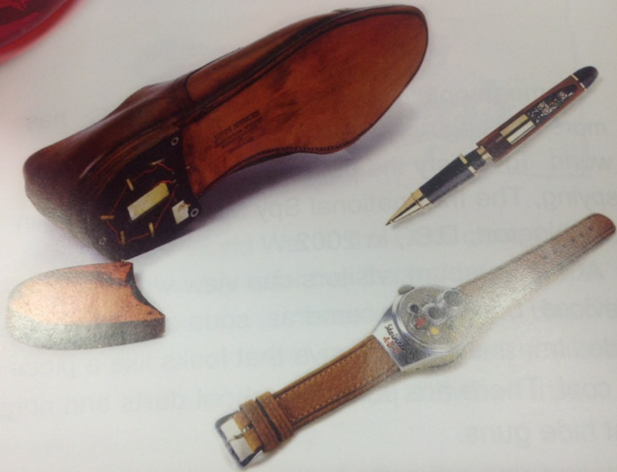
Tools spies have used to perform their work include a shoe and a pen with radio transmitters and a wristwatch camera.
